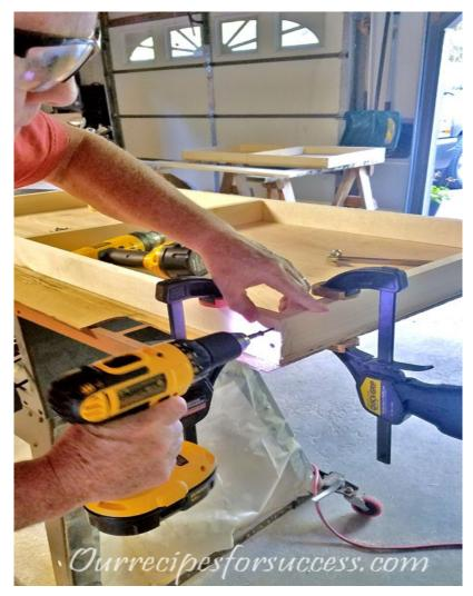
At this point it's time to add a little glue to the joints and screw the 1"x3" boards together. Make sure the screws are tight and the screw heads are slightly recessed into the countersink. Continue securing all the boards in the same fashion.
