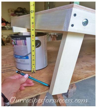
With the legs cut and attached, this is the best way we found to cut the legs to length. This method allows you to get the exact 12" height for the back of the cornhole board. It works best with a couple sawhorses and a piece of plywood at least 4' long.
