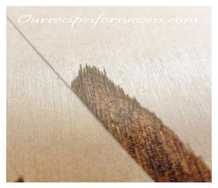
**Staining Tip** - If you are staining your boards, with a design, we would like to offer one very important tip. Before staining, score all the lines with a thin bladed razor bladed razor knife. This X-Acto knife from Amazon is a perfect example of what to use. You'll need to make the score lines at least 1/16" deep. These score lines will help prevent the stain from "bleeding". This will give you a nice clean line between two different colors of stain.
